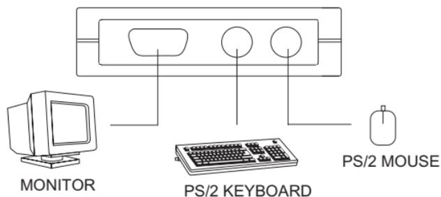
2. Use the KVM cables (as described in the Hardware Requirements section), to connect the monitor, keyboard and mouse ports of the computers to the CPU Ports (on the front and rear panels), as shown in the diagram below.
