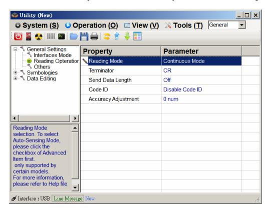
7. Click the Up Arrow on the Toolbar to upload configuration to the scanner and you are done!
